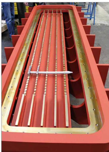
Ice-hardened hydrophone frame: manufactured in Germany (left) and ready to be installed (right)
