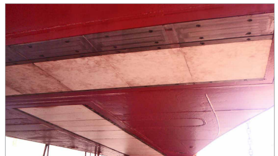
Mills cross installation of projector and hydrophone arrays
