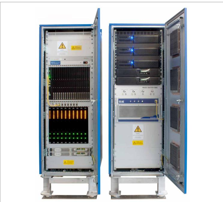
ELAC SeaBeam 3012 multibeam sonar electronics
