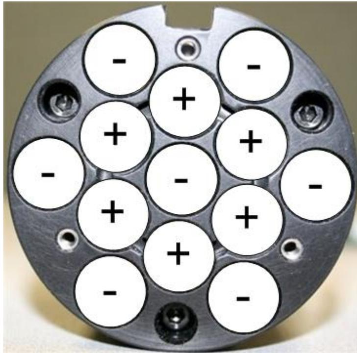
Figure 3 - BATTERY PACK CELL POLARITY
